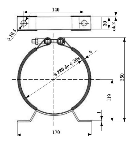
Clamping ring material - stainless steel Protective covering material - oilproof rubber Weight  $\sim 0.51\ kg$
