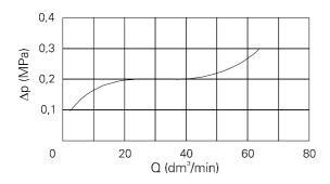
Pressure drop  $\Delta$  p in relation to flow rate Q with constant throttling
