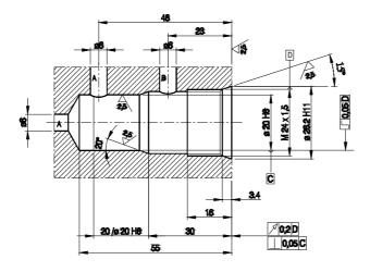
Seat dimensions ( torque for tightening the valve - 80  $\mbox{Nm}$  )
